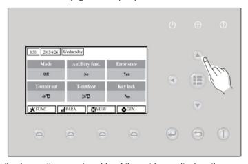
(6) Fully close the ball valve on the gas pipe side of the outdoor unit when the pressure gauge on the gauge manifold shows 0.05 to 0 MPa [Gauge] (approx. 0.5 to 0 kgf/cm²) and quickly stop the air conditioner. Then press UP key or Down key or ON/OFF key can exit pump down mode.
