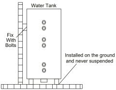
The minimum clearance from the water tank to combustible surface must be 500mm.
