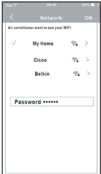
12. Select your own WiFi network, for example My Home (the picture is only for reference). 13. Enter your own WiFi router password and click OK.
