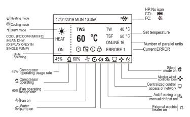
Set temperature:TWS/T5S:SETTING TEMPERATURE;TW:TOTAL OUTLET WATER TEMPERATURE, T5:TANK TEMPERATURE;TSF:SAFE TEMPERATURE;
