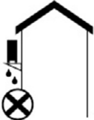
The manufacturer does not recommend mounting the device on the building facade.
