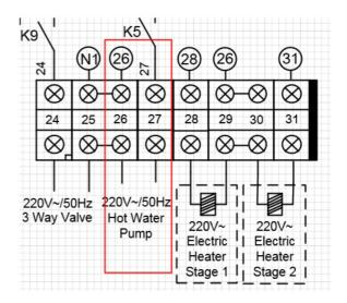
0 – Charging pump for domestic hot water tank. Pump used in the case of an additional heat exchanger between the unit and the DHW tank, separating the circuits.
