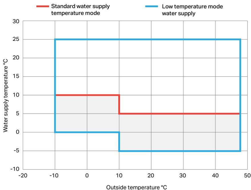
In cooling mode, it operates effectively in external air temperatures ranging **from -15°C to +48°C**, offering a **stable supply water temperature of up to +25°C**, which enables operation in advanced air conditioning systems, including active floor or ceiling cooling installations.
