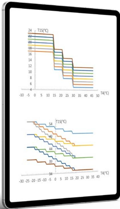
The heat pump uses a **weather curve** function that **automatically adjusts the temperature of the medium in heating or cooling mode to the changing outside air temperature, which affects:**
