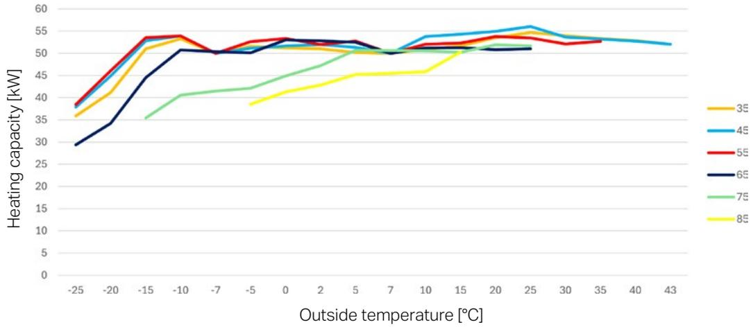
Performance chart of the KCOP060PMA3 heat pump in heating mode for selected water temperatures (35, 45, 55, 65, 75, 85 °C)
