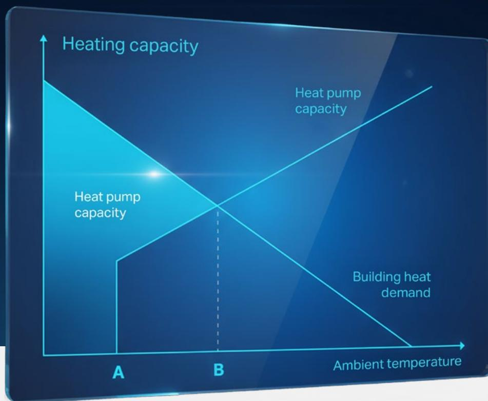
The controller enables **hybrid system** management, ensuring flexible and economical cooperation between the heat pump and an external heat source, such as a boiler or district heating network.
