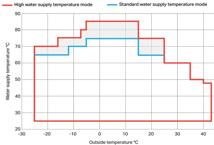
The KCOP Arctic Power heat pump guarantees thermal comfort regardless of weather conditions. Designed to operate in extreme temperatures, it provides **reliable heating from -25°C to +43°C**, supplying heating water at temperatures up to **85°C**, which allows for effective cooperation with traditional radiator installations, especially in modernized buildings.
