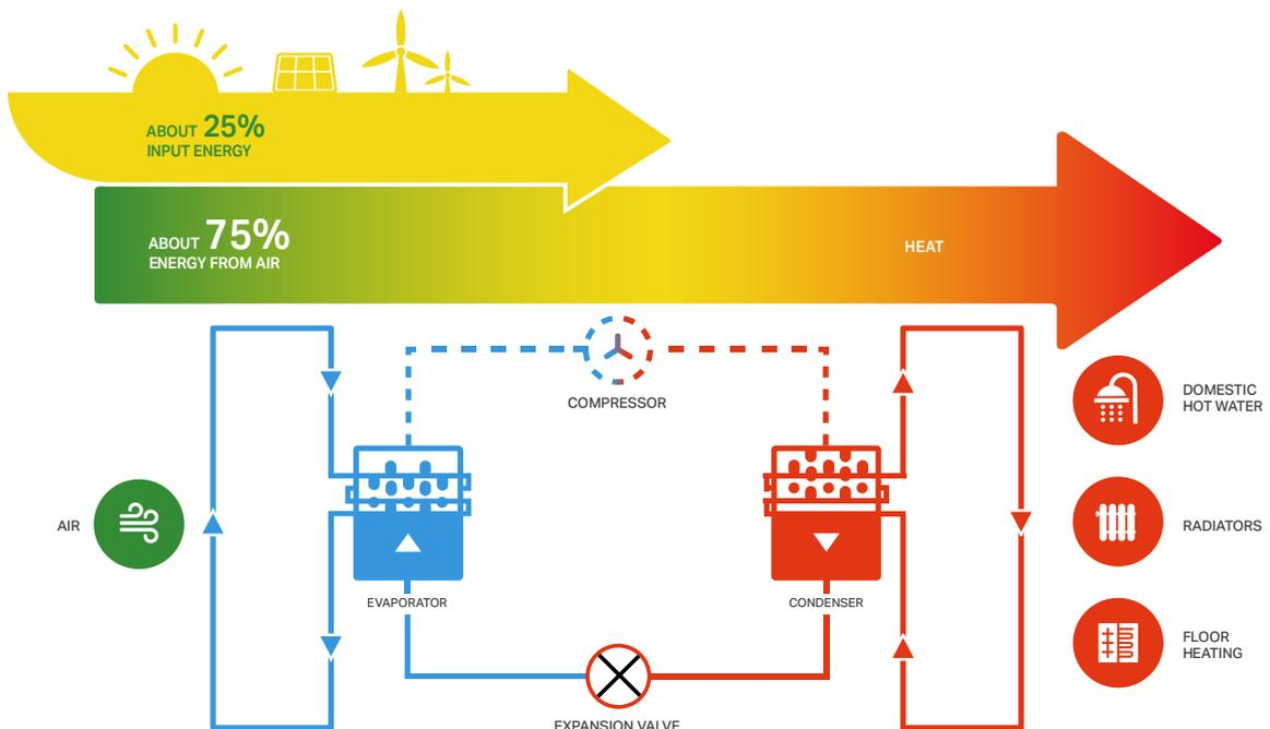
Kaisai heat pumps are highly efficient – for every unit of electricity consumed, they can deliver between 3 and 5 units of heat. This makes them one of the most economical and environmentally friendly ways to heat buildings.
