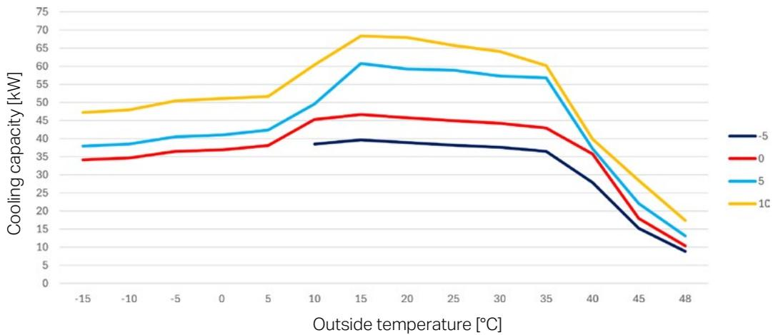
Performance chart of the KCOP070PMA3 heat pump in cooling mode for selected water temperatures (-5, 0, 5, 10°C)
