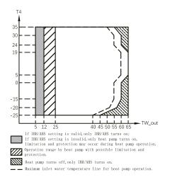
In DHW mode, the water flowing temperature(TW\_out) range in different outdoor temperature(T4) is listed below:
