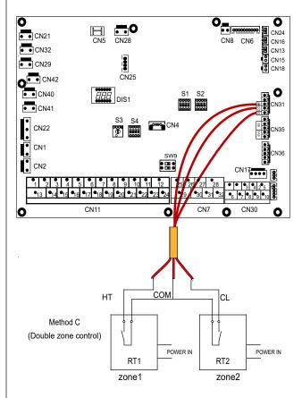
There are three methods for connecting the thermostat cable (as described in the picture above) and it depends on the application.
