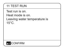
During HEAT MODE test running, the default target outlet water temperature is 35°C. The IBH (internal backup heater) will turn on after the compressor runs for 10 min. After the IBH runs for 3 minutes, the IBH will turn off, the heat pump will operate until the water temperature increase to a certain value or the next command is received.
