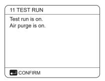
When in air purge mode, SV1 will open, SV2 will close. 60s later the pump in the unit (PUMPI) will operate for 10min during which the flow switch will not work. After the pump stops, the SV1 will close and the SV2 will open. 60s later both the PUMPI and PUMPO will operate until the next command is received.
