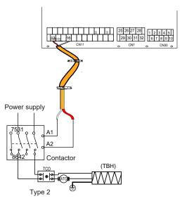
Control signal port of indoor unit: The CN11/CN7 contains terminals for solar energy, 3-way valve, pump, booster heater , etc.
