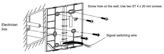
Screw hole on 86 electrical box; Use two M 4 x 25 mm screws
