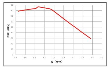
Available external static pressure VS Flow rate
