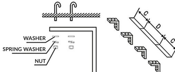
**4.3.3** Set the mounting plate on the ceiling brackets and ensure safe & fixing (use the bolts attached to the ceiling brackets as Fig). Using the ceiling brackets to hang from the ceiling, the position of mounting plate can be adjusted in the limit of 100mm.
