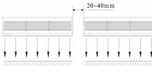
**3.5** Don't allow gaps between the unit and the wall. When hanging it from the ceiling, using the enclosed ceiling braskets.
