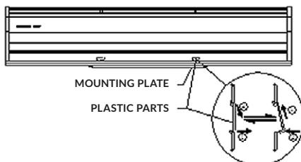
**4.1.2** Fix the bolts in the proper position (decide the position with the mounting plate and pour cement into the bolt holes).
