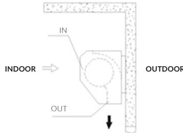
**3.3** Don't install the unit too low, no less than 2.3 meter from the ground.
