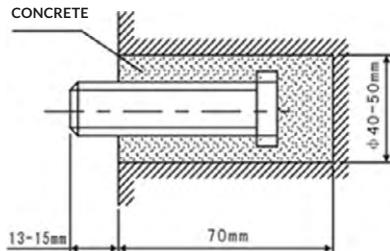
**4.1.3** When the cement has freeze, fit the mounting plate (use the washer and nut according to the following).
