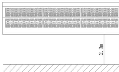
**3.4** When the entrance is wider than the unit, it is recommended to install two or more units in parallel. In this case, provide 20-40mm gaps between the units.
