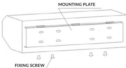
**4.3.2** Fixing ceiling brackets as Fig.
