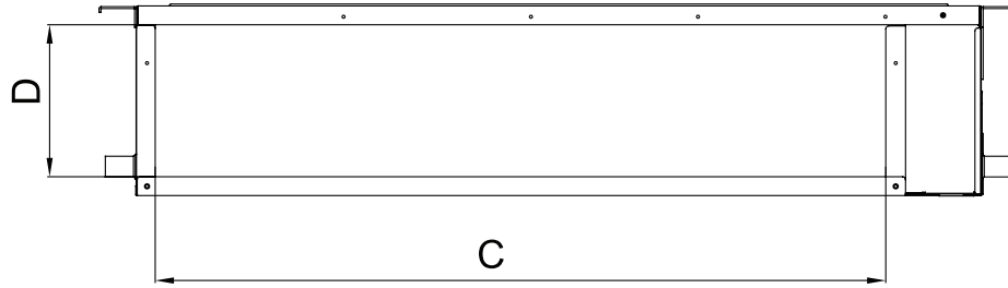
Fig.35 Return Air Inlet
