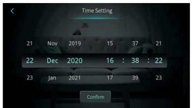
When entering the page of system time setting, the system time will be initialized to the time at the moment when the system time setting button is pressed, and you can adjust the time by sliding up and down. Note: When the temperature unit is? the time format is displayed as: month-day-year hour: minute: second.
